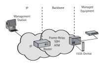
Most of the described maintenance and management mechanisms below use IP as the underlying protocol to communicate with the Telindus equipment. Some units (such as the router range) have a direct IP Ethernet port, whilst other units (such as the Aster and Crocus modem ranges) are connected through a controller device (1035 Orchid) which acts as an IP proxy device.
